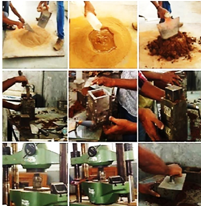
Fig.2: Casting of Cube Specimens
