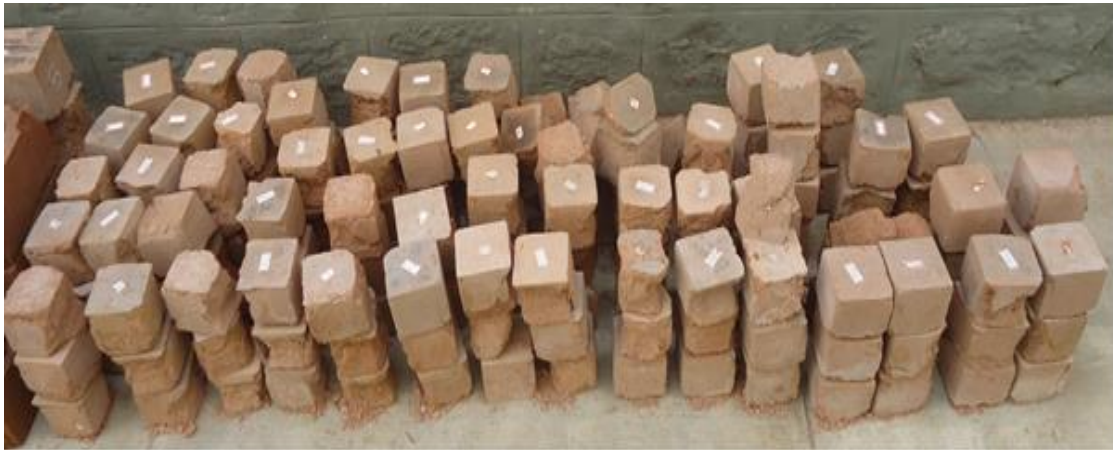
Fig.3: Cubes stacked after compressive strength test
